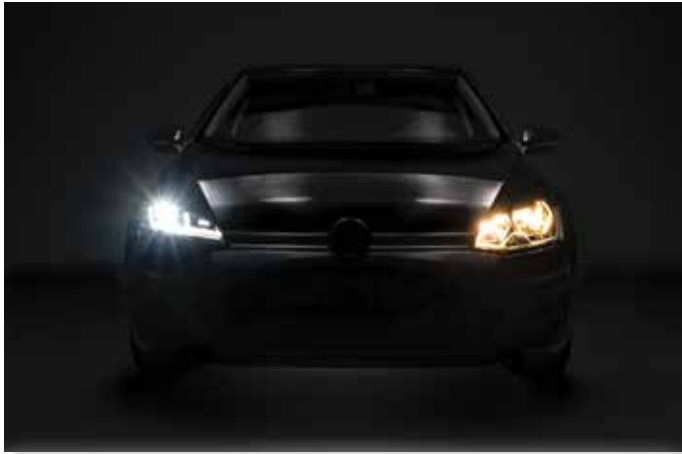
The LEDriving headlamp for the VW Golf VII (left) compared to the original halogen version (right).
